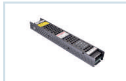
HLD-4871 (150W - 24V) 0/1-10V + Triac Dimmable AC170-250V / 1.2A/110VAC
